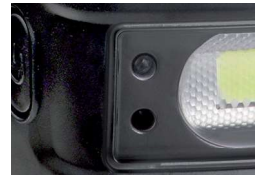
Move your hand in front of the sensor: it turns on and off. No need to touch it
